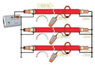
The user must only verify the display. This means, that generally, only one conductor or cable has the correct polarity while all other cables have the opposite polarity.
