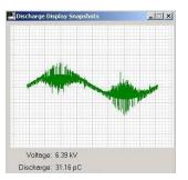
Fig. 1: Surface PD activity on an 11kV circuit breaker. Low discharge amplitude, high discharge rate
