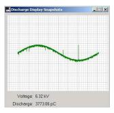
Fig. 2: Internal PD activity on a 10kV current transformer. High discharge amplitude, low discharge rate
