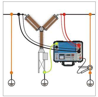
You can make tests with both sides of the test object grounded, an additional safety feature.
